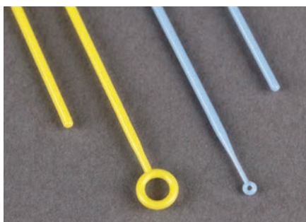
Loops feature integrated needle at reverse end
