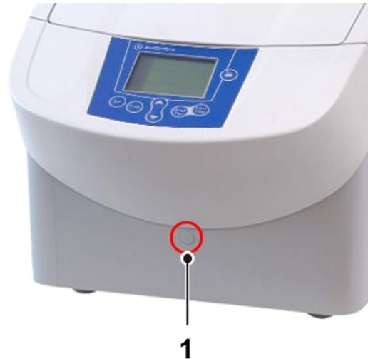
Fig. 10: Position of the opening for the emergency lid release
