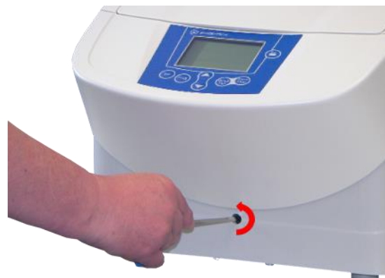
Fig. 11: Manual release of the lid lock
