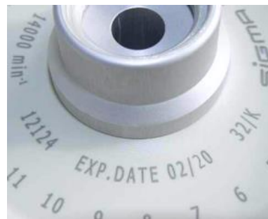
Fig. 4: Different service life – engraving on the bucket/rotor
