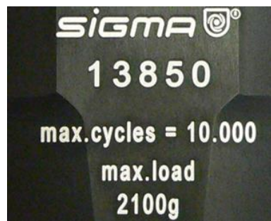
Fig. 4: Different service life – engraving on the bucket/rotor
