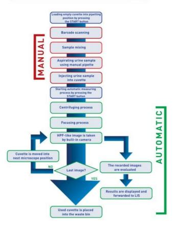
The operation of this analyzer is based on the patented UriSed Technology, which is actually the automation of traditional manual microscopy. The operator only needs to load a special disposable cuvette and inject native urine sample into it using a manual pipette. Working without any special liquid reagents, UriSed mini performs all the rest automatically.
