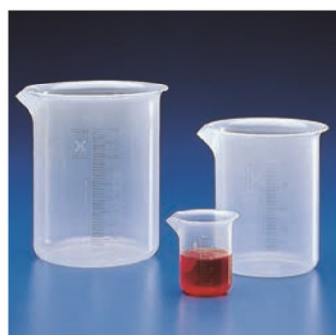
Polypropylene (PP) with Molded Graduations
